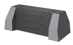
Specifications – H-Block Support Material - 100% recycled rubber, UV resistant The HBS-Base Series is UV resistant and suitable for installation on most types of roofing material or other flat surfaces. Can be used as a curb (sleeper) replacement. Screw fasteners can be used to attach one or two hole pipe straps or a piece of strut (not included).
