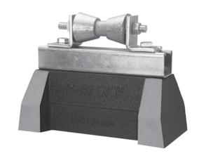
Specifications – HBS-Roller Series H-Block Support with: 1%" H-132 Channel Material - 100% recycled rubber, UV resistant Pipe O.D. - 1" thru 10" The HBS-Roller Series is designed for superior support of natural gas and refrigeration pipes. The roller allows for longitudinal movements of the pipe. This support is suitable for most types of roofing material or other flat surfaces.
