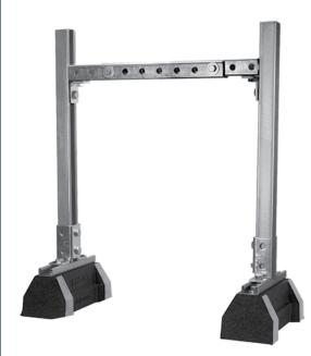
Specifications – HBS-DSAW Adjustable Width & Height. All hardware required for assembly is included. Base Material - 100% recycled rubber, UV resistant Telescopic Crossbeams - 15/11" H-132-RS3 Channel The HBS-DSAW Series is designed specifically for supporting duct work. The telescopic cross beam provides easy size adjustments. A wide range of support widths are provided from  $19\frac{1}{4}$ " to  $103\frac{5}{8}$ "
