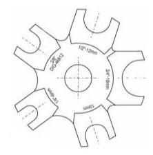
On initial assembly, apply no-go gap inspection gauge to make sure that the make-up distance is sufficiently pulled-up.
