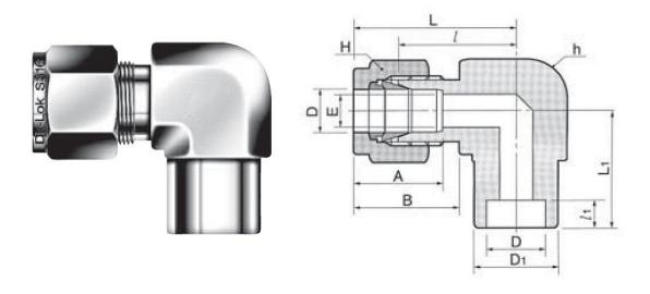
**Connects fractional tubes Classification: Tube to Weld End**
