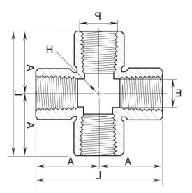
**End Connection**: All 4 end connections are the equivalent pipe size with female NPT threads. **Series**: Standard High Pressure Instrumentation Threaded Fittings
