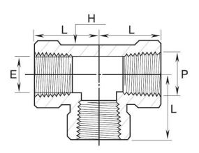
End Connection: Female NPT x Female NPT x Female NPT Series: Standard High Pressure Instrumentation Threaded Fittings
