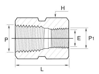
**End Connection**: Female NPT to Reduced Female NPT Threads **Series**: Standard High Pressure Instrumentation Threaded Fittings
