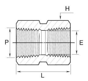
End Connection: Female NPT to Equal Female NPT Threads Series: Standard High Pressure Instrumentation Threaded Fittings
